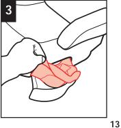
Cup Holder Insert (on select models): Cup holder may have a removable liner for cleaning. To remove, pull up on corner of rubber insert and remove. Clean with a mild soap and warm water. When dry, replace insert.
